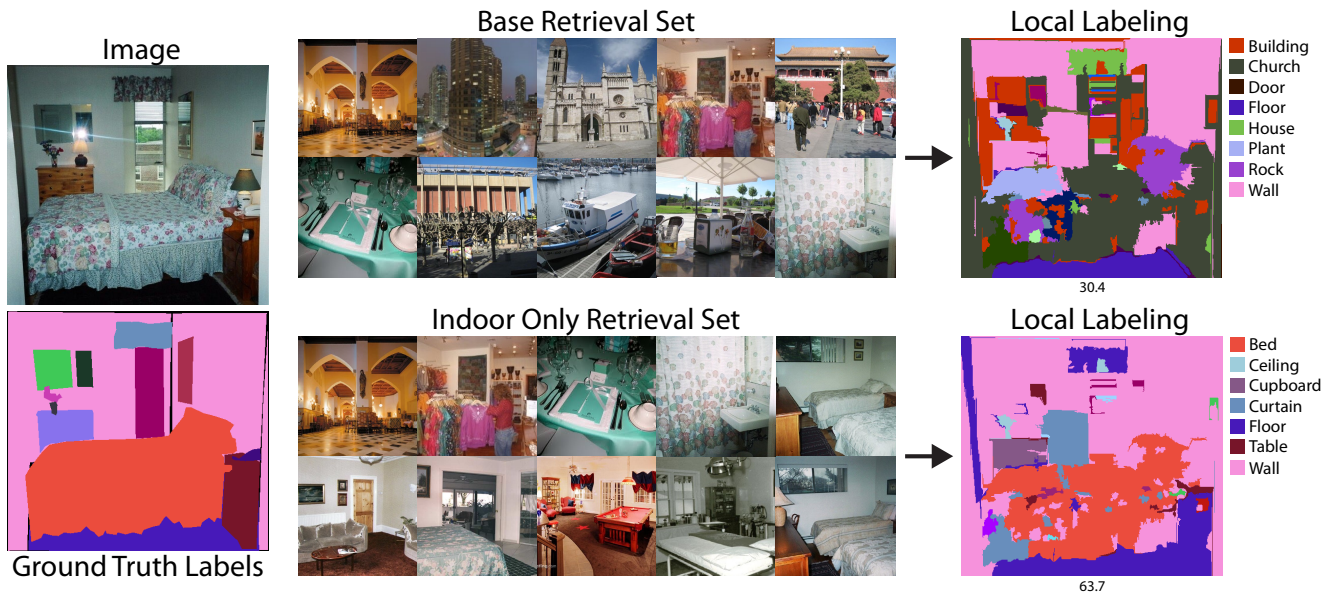
Fig. 6 Effect of drawing the retrieval set from the entire training set (“base retrieval set”) vs. drawing it from the correct scene type (“indoor only retrieval set”). With the base retrieval set, the local labeling result has a mix of indoor (floor, wall) and outdoor (building, rock) classes. On the other hand, if we restrict the retrieval set to consist only of indoor images, we get a much cleaner result – in particular, we manage to label most of the bed.
